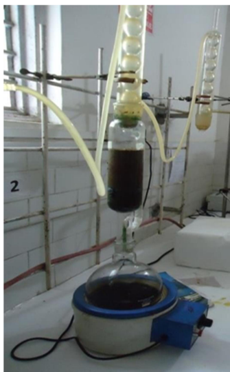
Figure : Soxhlet apparatus
