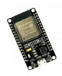
ESP32 based boards come in a variety of shapes and sizes and pinout of each board is different to other. Also, not all pins of the ESP32 Microcontroller SoC will be available on a development board as some pins might be permanently tied to a dedicated function.
