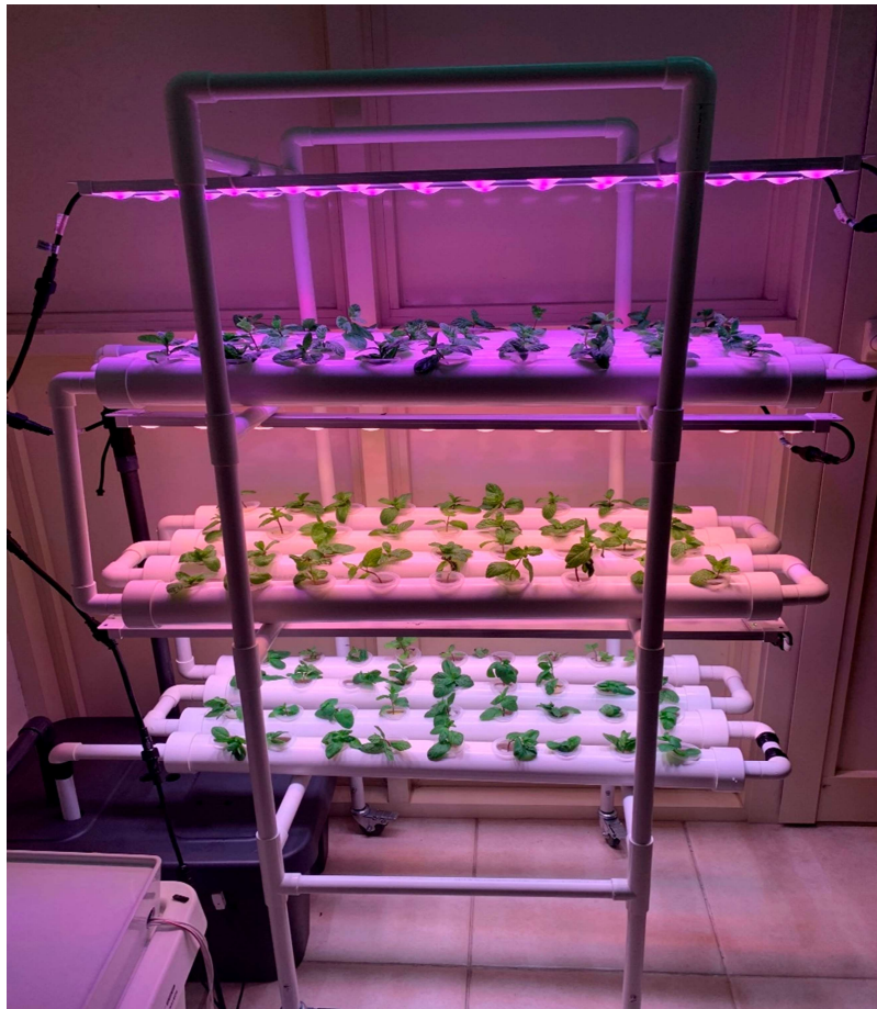
Figure 3. Vertical NFT hydroponic structure assembled and connected to the monitoring and control system.
