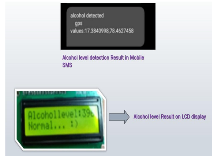
Fig: -16 Results on LCD & SMS to Phone
