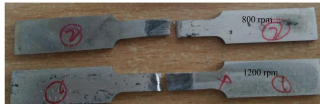
**Figure 2.**The fracture location of the tensile specimens' joints welded at rotation speed of 800 rpm and 1200rpm
