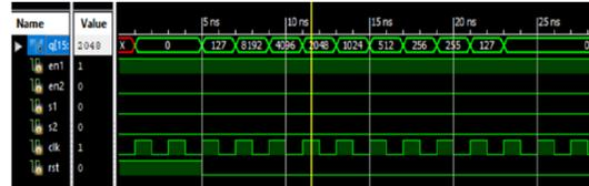
**Fig:5 Simulation results of LFSR**
