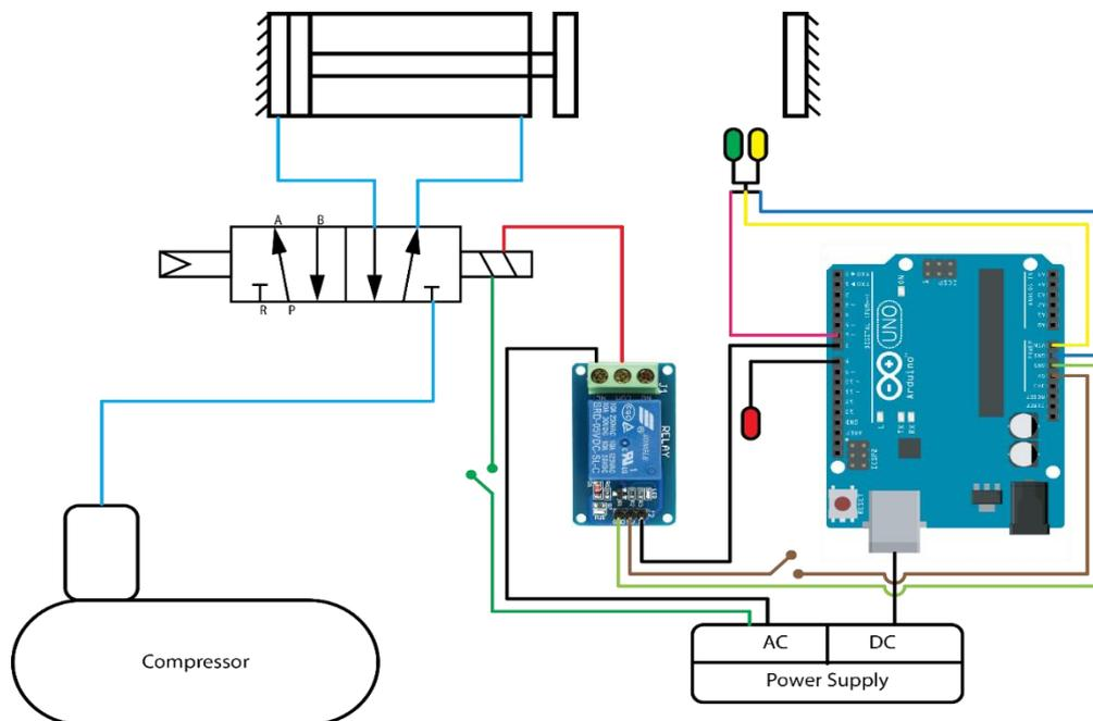
Figure 1: Pneumatic vice circuit diagram
