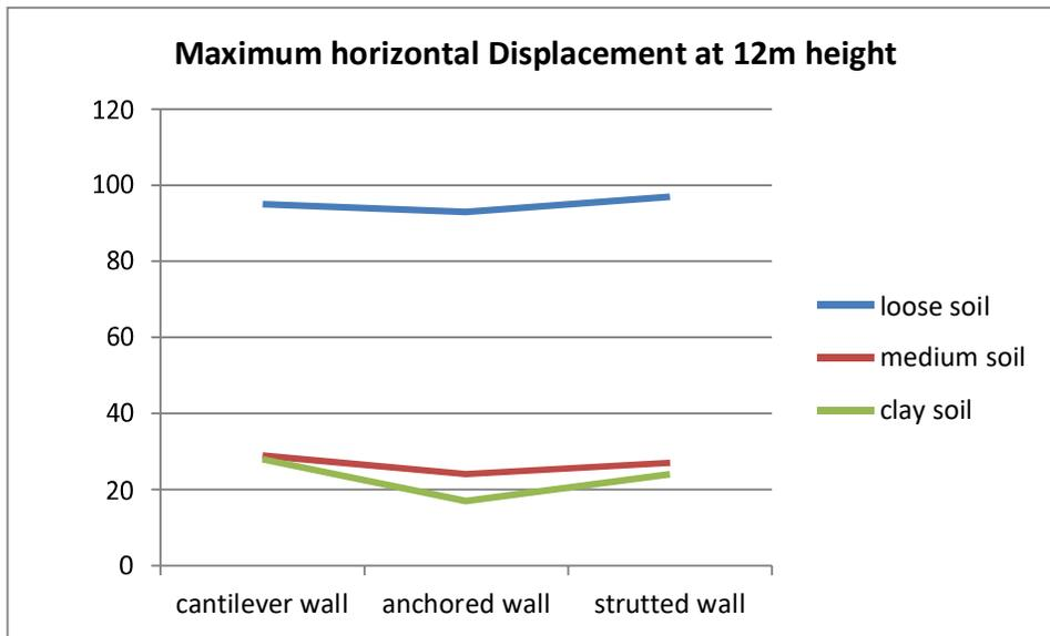
Figure 4.5 Maximum horizontal displacement of the diaphragm wall with different diaphragm wall (Case 3)
