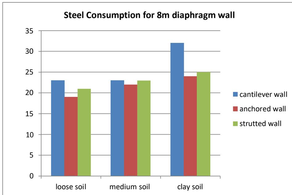
Figure 4. 4 Steel Consumption of different diaphragm wall (Case 2)
