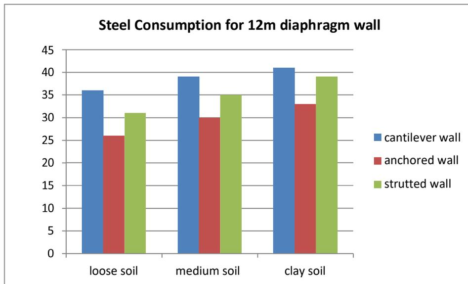
Figure 4. 6 Steel Consumption of different diaphragm wall (Case 3)
