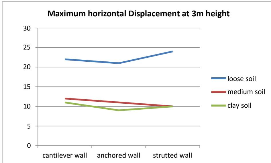
Figure 3.1 Maximum horizontal displacement of the diaphragm wall with different diaphragm wall (Case 1)
