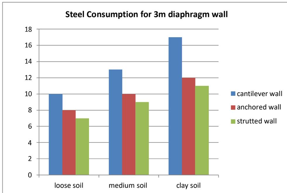
figure 3. 2 Steel Consumption of different diaphragm wall (Case 1)
