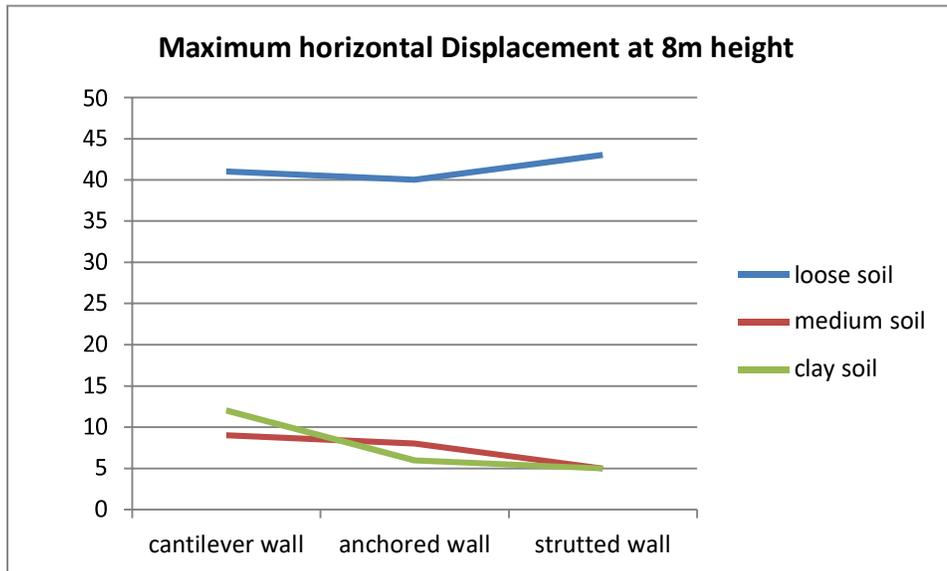
Figure 3.3 Maximum horizontal displacement of the diaphragm wall with different diaphragm wall (Case 2)
