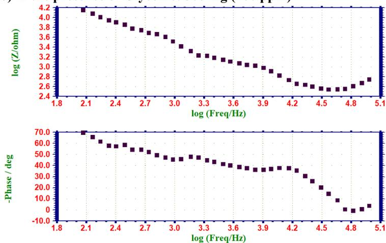
**Figure 7: AC impedance spectra (Bode Plots) of Ni–Ti alloy immersed in Artificial Saliva (AS) in the presence of Zinetac150 mg (100 ppm)**
