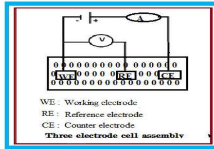
Figure 1: Three electrode cell assembly
