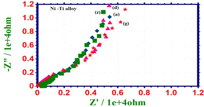
Figure 3: AC impedance spectra (Nyquist Plots) of Ni –Ti alloy immersed in Artificial Saliva (AS) in the absence of Dolo650 mg, Glycomet 500 mg and Zinetac150 mg
