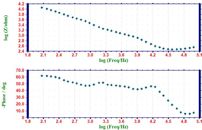
Figure 4: AC impedance spectra (Bode Plots) of Ni –Ti alloy immersed in Artificial Saliva (AS) in the absence of Dolo650 mg, Glycomet 500 mg and Zinetac150 mg
