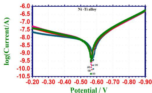
Figure 2: Polarization curves of Ni –Ti alloy immersed in Artificial Saliva (AS) in the absence and presence of Dolo650 mg, Glycomet 500 mg and Zinetac150 mg
