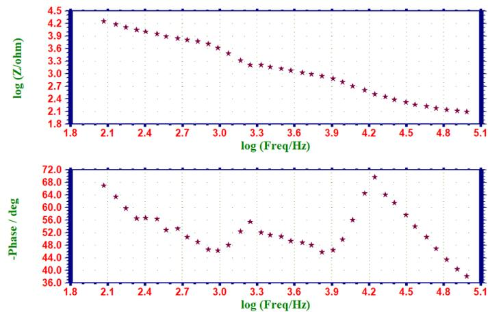
**Figure 6: AC impedance spectra (Bode Plots) of Ni–Ti alloy immersed in Artificial Saliva (AS) in the presence of Glycomet 500 mg (100 ppm)**
