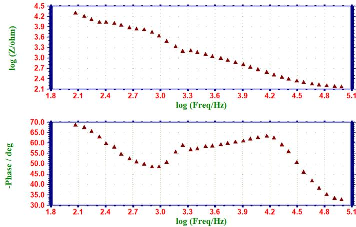
**Figure 5: AC impedance spectra (Bode Plots) of Ni–Ti alloy immersed in Artificial Saliva (AS) in the presence of Dolo650 mg (100 ppm)**
