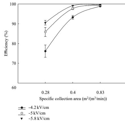
(b) Total collection efficiency versus SCA in the wet ESP
