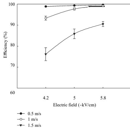
(a) Total collection efficiency in the wet ESP
