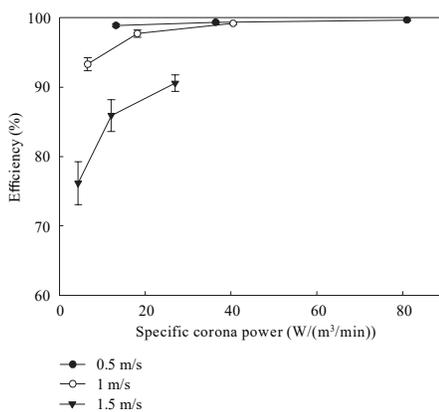
(c) Total collection efficiency versus specific corona power in the wet ESP
