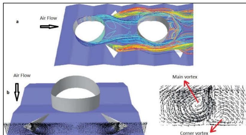
**Figure 4. (a) Streamlines starting from the first row tube and delta winglets. (b) Secondary velocity vectors at the cross-section of  $x = 21$  mm downstream of the first row delta winglet in wavy fin channel with in-line tube array.**
