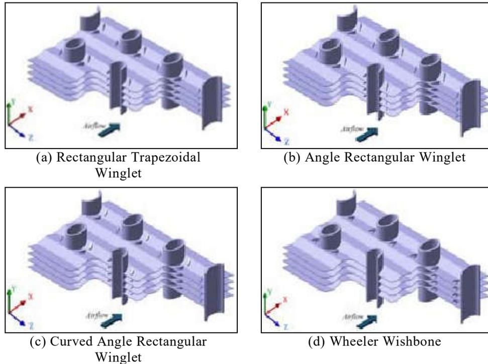
**Figure 1. Isometric aligned section of core region of a smooth wavy fin-and-elliptical tube bank with mounted VGs.**
