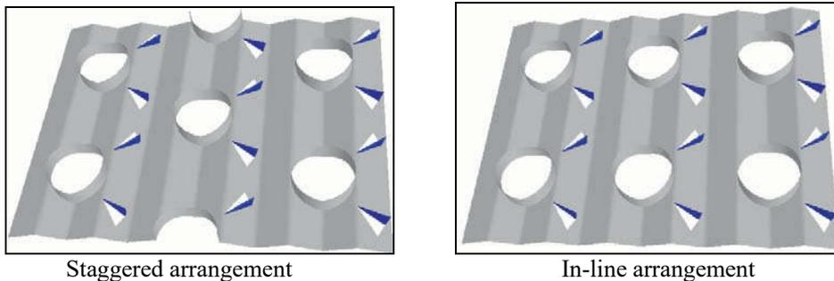
**Figure 3. Schematic view of a wavy fin with delta winglets.**
