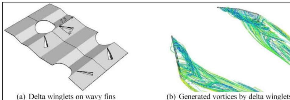
**Figure 2. Delta winglets and vortices generated alongside the wavy fin-and-tube heat exchangers.**
