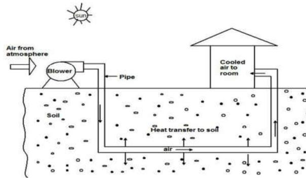
Figure 1: Two-dimensional EAHE model
