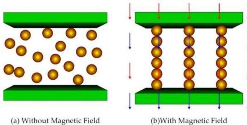
**Figure 1.1 Working Principle of MR fluid [1]**
