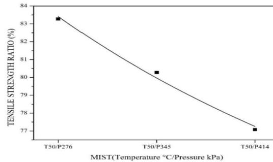
**Figure Number 8. Variation of TSR at 50 °C for different pressures in MIST conditioning for the mix with Evotherm**
