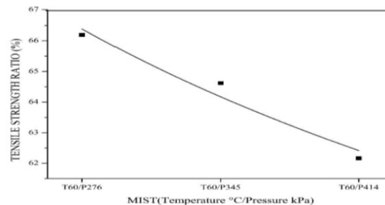
**Figure Number 6. Variation of TSR at 50 °C for different pressure in MIST conditioning for the control mix**
