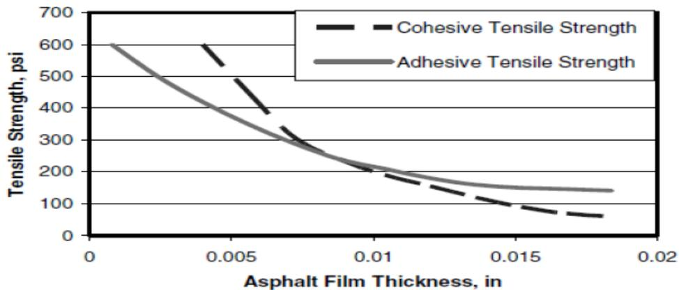
Figure Number 1. Adhesive Vs. Cohesive bond failure in bituminous mixes (Source: Cheng et al. 2002)
