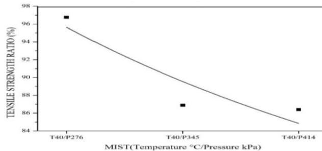
**Figure Number 7. Variation of TSR at 40 °C for different pressures in MIST conditioning for the mix with Evotherm**
