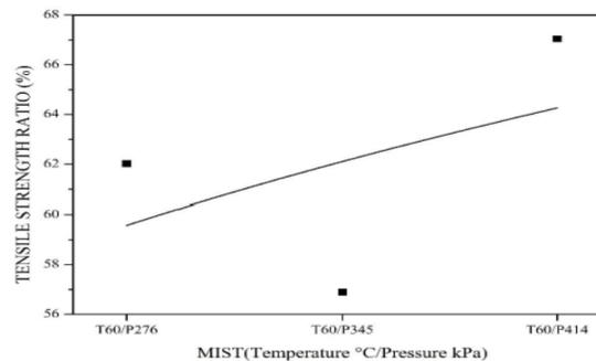
**Figure Number 9. Variation of TSR at 60 °C for different pressures in MIST conditioning for the mix with Evotherm**
