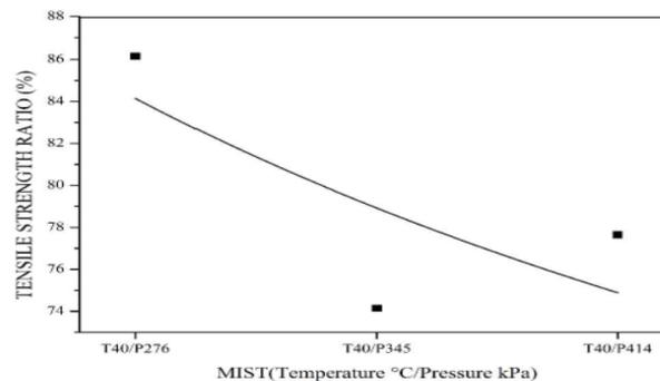
Figure Number 4. Variation of TSR at 40 °C for different pressure in MIST conditioning for the control mix
