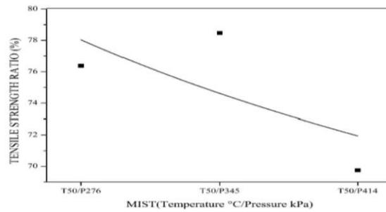
**Figure Number 5. Variation of TSR at 50 °C for different pressure in MIST conditioning for the control mix**
